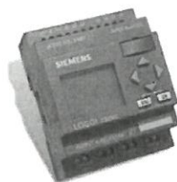
The programmable logic unit is the brain of the MVP-Duplex control panel
