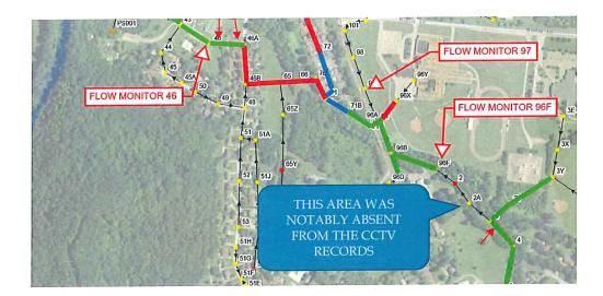
For each video, First Response provided a pipeline summary sheet. Each of these reports were compared to notes taken during the CCTV review, and for the most part the data was in sync. A sample pipeline report is shown below (note, this segment should have been called out as having excessive grease buildup to the point that the camera had trouble passing):
